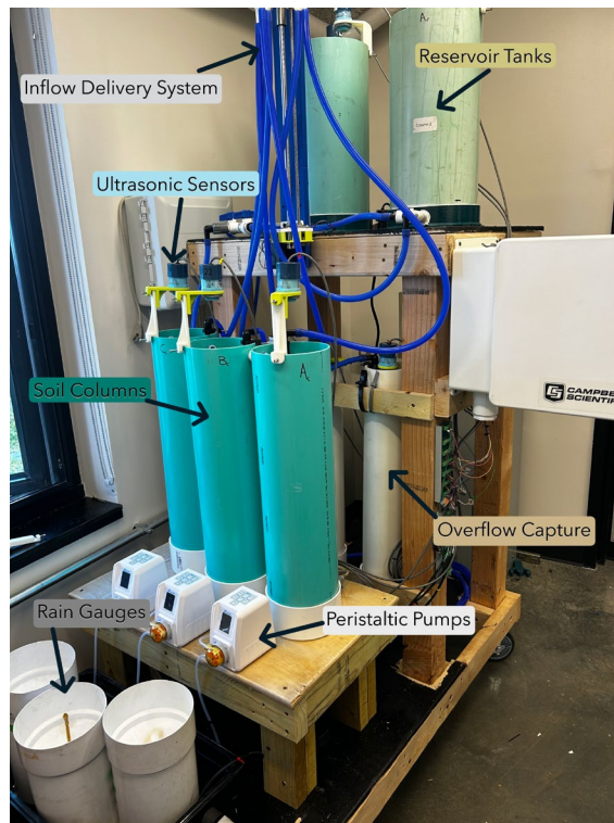
Figure 2. Experimental setup with three soil column replicates, inflow delivery system, and outflow measurement.
